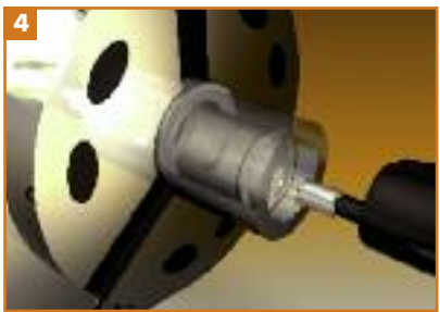
Retraction in X and Z direction
